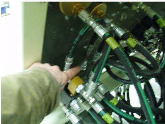
11. Spike relief adjustments must be made to the 3 lever valve bank:
