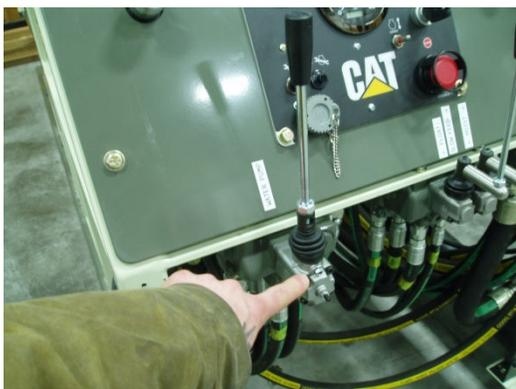
6. Adjust two set screws on Kawi pump:
